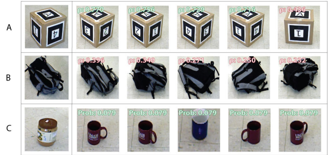
Fig. 6. Sample queries from the experimental test set that resulted in failure. In Query A, we show an aspect comparison failure with an ARcube where the correct box orientation is returned but the alphanumeric labels are incorrect. This is likely because distinguishing between characters did not help on the ILSVRC data set and therefore individual characters are not encoded in \bar{\Lambda} . Query B shows an aspect comparison failure case involving a deformable object, where the backpack has been emptied and the straps appear in different orientations. Query C shows one of the few class identification failures where a jar of peanut butter previously unseen by the model database is incorrectly identified as a class of cup.
