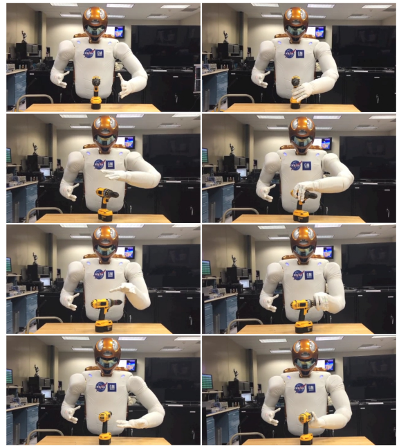
Figure 3: Robonaut 2 grasping the drill posed at different orientations. Image pairs in the same row represents the intermediate and final states of one drill grasping trial.
