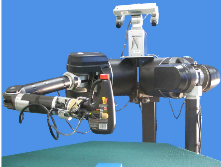
Figure 4.3. Each of Dexter’s arms has 7 DOF and is equipped with a three-fingered hand with four total degrees of freedom. The stereo head has four degrees of freedom.
