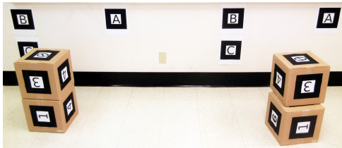
Figure 4: On the left is the demonstrated stack, while the right stack is the approximate copy constructed by the robot.
